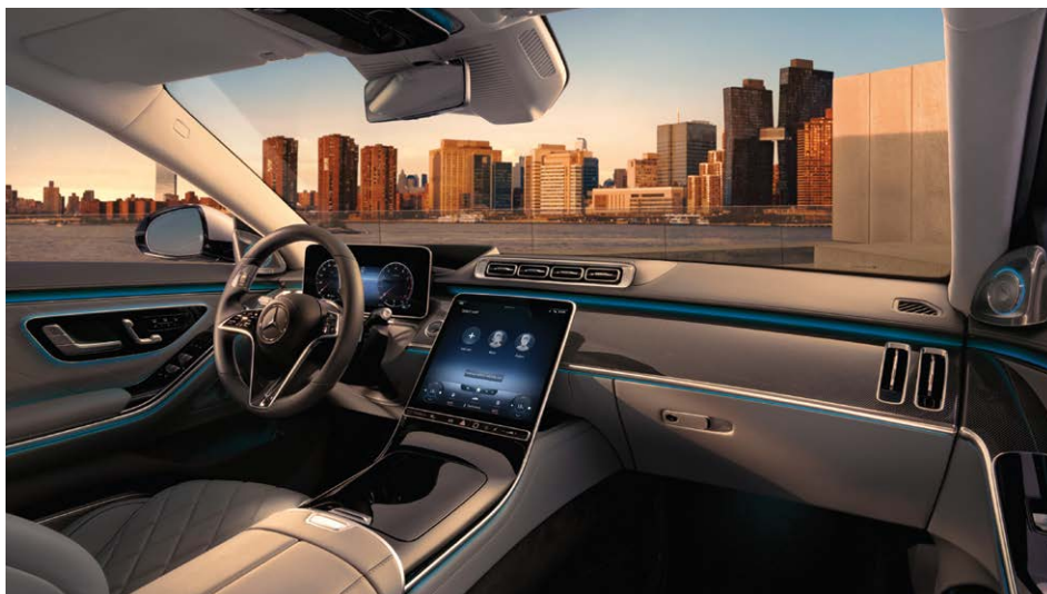
The second-generation Mercedes-Benz User Experience (MBUX) defines the car-driver interface via up to five large displays. The central OLED can display a 3D overhead view of the car and its surroundings to ease tight manoeuvring
